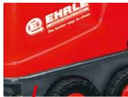
Corrosion proof powder coated steel chassis with impact resistant protective plastic cover
