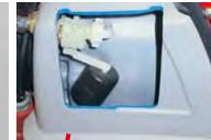
The rotation molded chassis is hollow and serves as water storage tank (35 I) and buffer was well as water supply separation
