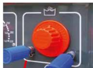
Control valve for continuous addition of detergents
