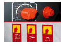
Level 2 - OUTSIDE - comprising for use of the operator: a main switch and two ON/OFF switches for hot water and detergents. Preset parameters can not be changed from the outside.
