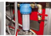
Largely dimensioned water inlet filter
